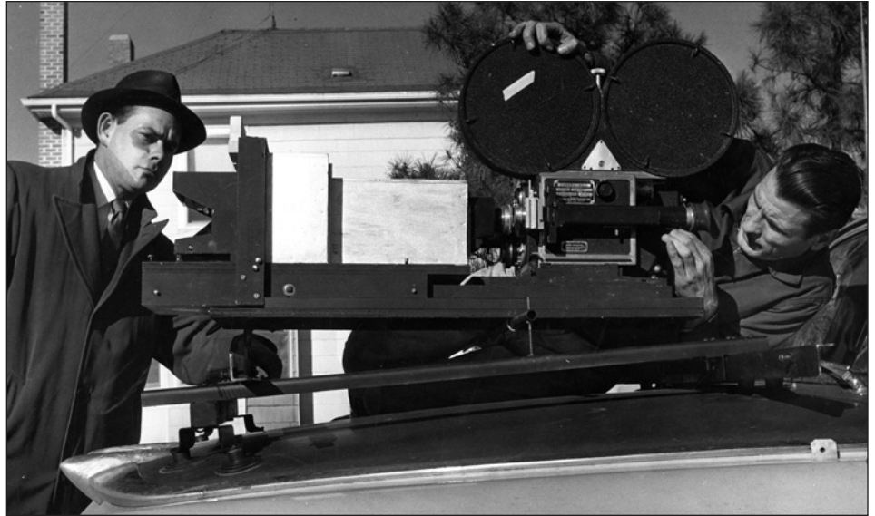
Rowe Carney Jr., left, and Tom Smith check the camera attached to Carney's car. Through experimentation, the pair created a system of lenses, mirrors, and other equipment that could capture a 180-degree view and then project it from one reel of 35mm film onto a special screen.
