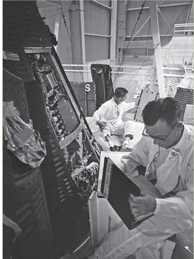
In this photo taken by St. Louis Post-Dispatch photographer Art Witman during Gemini's launch preparations, McDonnell technicians at Kennedy Space Center review spacecraft hardware in the Gemini equipment section.
